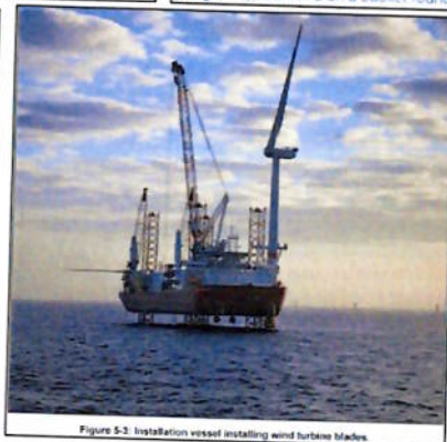
Figure 5-3 Installation vessel installing wind turbine blades
